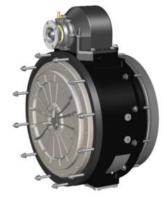
The overall system provides uninterrupted motion transmission from the engine through the main transmission clutch pack. The PTO on the top can be engaged/disengaged through hydraulic control.
